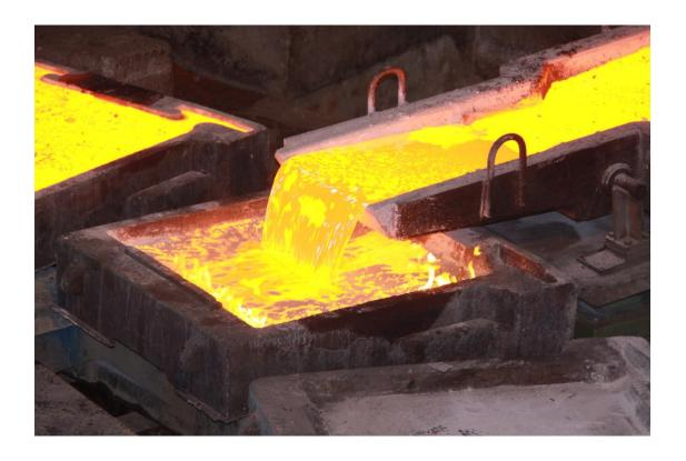
(Anode copper plate pouring scene and anode plate)
