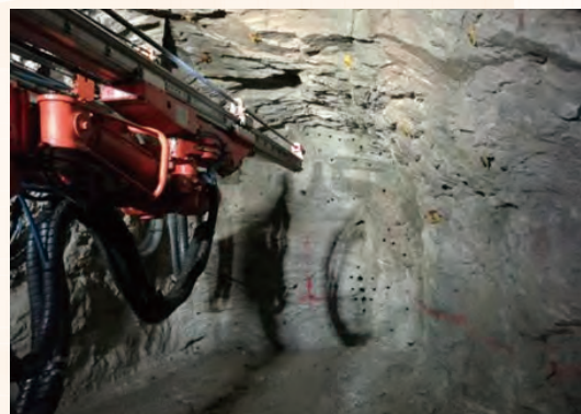
Underground simulative production training—DD422 idrilling jumbo conducts drilling
