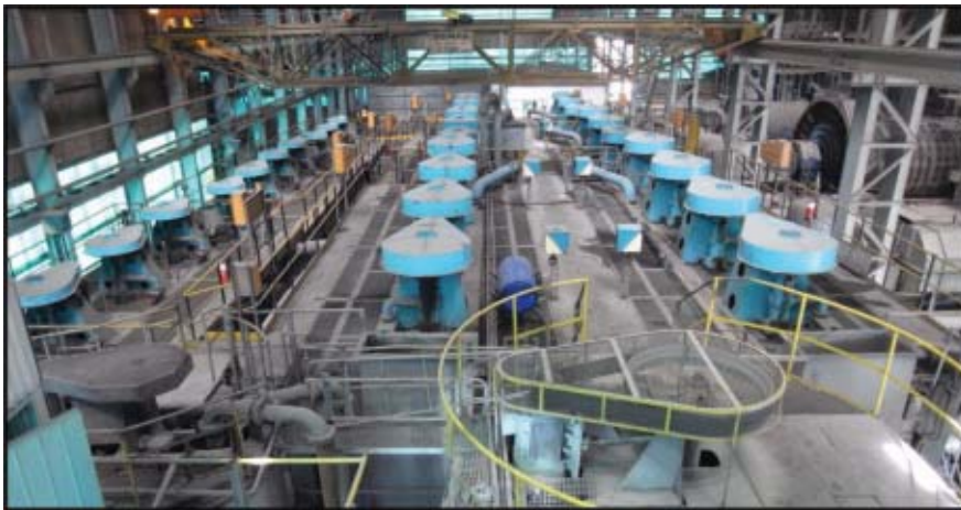
Figure 8-3: Flotation Section of the Chambishi Concentrator
