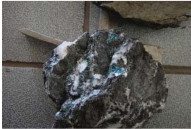
Figure 6-10: Bornite Mineralization in Fresh Sample — Chambishi Main
